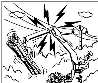
**NOTE: Failure to respect the minimum safe distances may result in electrical hazards for the operator and his assistants.**
