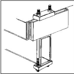
Check the tightening torque of the fixing rods of the crane.
