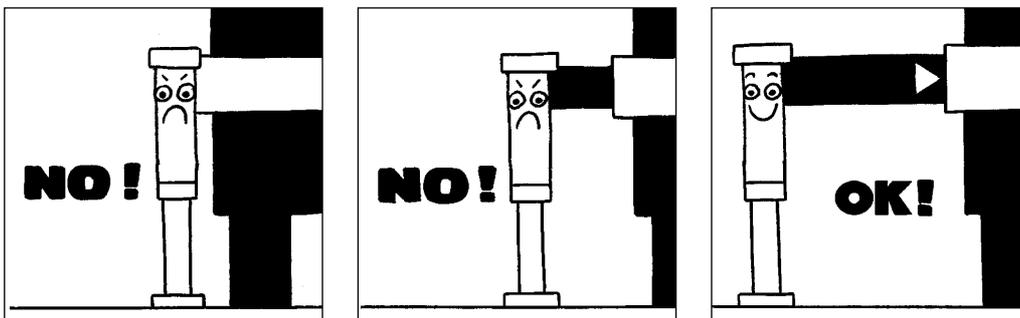
Level the crane so as it is always operated on a horizontal plane; check that the angle of inclination of the vehicle always does not exceeds five (5°) in any direction.
