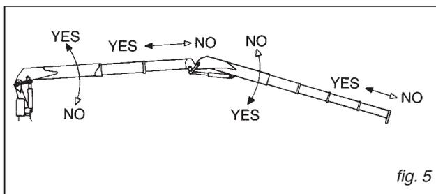
The lifting moment limiting device prevents the following manoeuvres:
