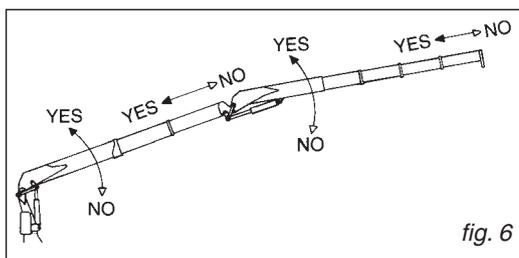
The crane configurations (fig. 5-6) indicate the manoeuvres which are allowed and not allowed by the device, in connection with the horizontal position of the crane and extension outer booms. When the moment is reduced, it resets automatically (the manoeuvres blocked by the device are released).
