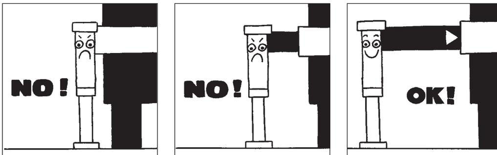
Stabilize the vehicle on a horizontal plane with a maximum tolerance of 1,5 degrees.
