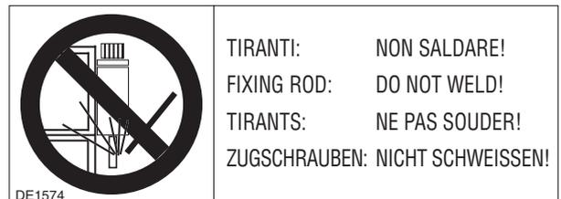
Do not weld the fixing rods of the crane (DE1574 fig. 19).
