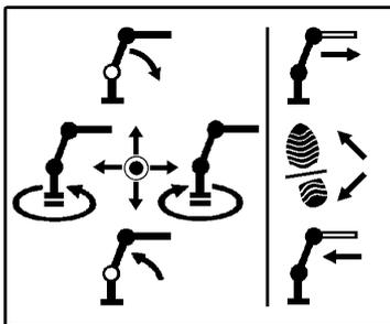
The joystick controls the **inner boom** and the **rotation** of the crane:
