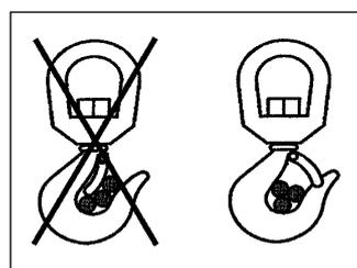
Check the efficiency of the hook safety catch.
