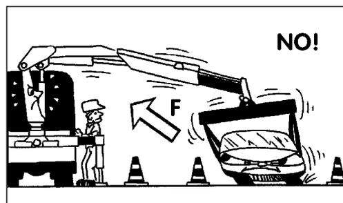
Do not utilize the crane for pushpull, lateral or sideways operations.
