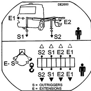
The extension and re-entering of the support and outrigger rams indicated on the fig. 9-10 coincide with what indicated on the plates **DE2600** and **DE2601** placed next to the control stations.
