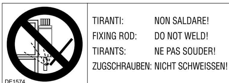
Do not weld the fixing rods of the crane (DE1574 fig. 17)
