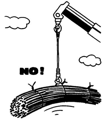
It is absolutely prohibited to walk or stop under a suspended load and for unauthorized persons to be within the working area.
