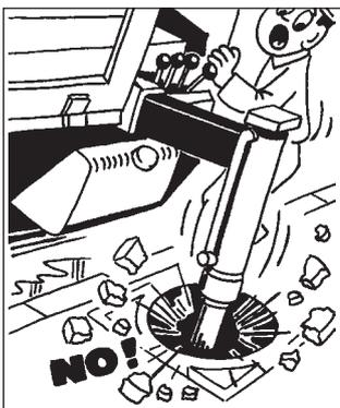
Never operate the outriggers when the crane is loaded.
