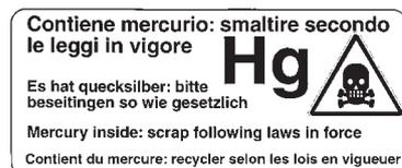
**MERCURY IS EXTREMELY TOXIC. IN CASE OF REPLACEMENT AND/OR SCRAPPING, DISPOSE OF OR RECYCLE THE CAPSULE CONTAINING MERCURY WITH MAXIMUM CARE, AND IN ACCORDANCE WITH THE NATIONAL REGULATIONS IN FORCE.**
